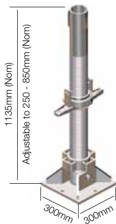
Acrow Powershore Adjustable Base Code: APSSJ Wt: 51kg
