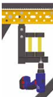
FASTENED BY SCREWS 6 X 60 DIN-7505-A
