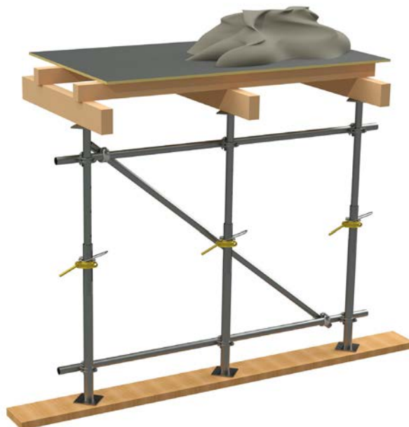
USING BRACING FOR FALSEWORK STABILITY
