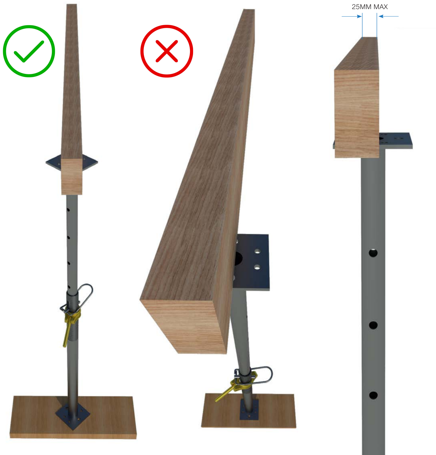
BEARER SHOULD BE PLACED AND NAILED INTO THE CENTRE OF THE INNER TUBE END PLATE
