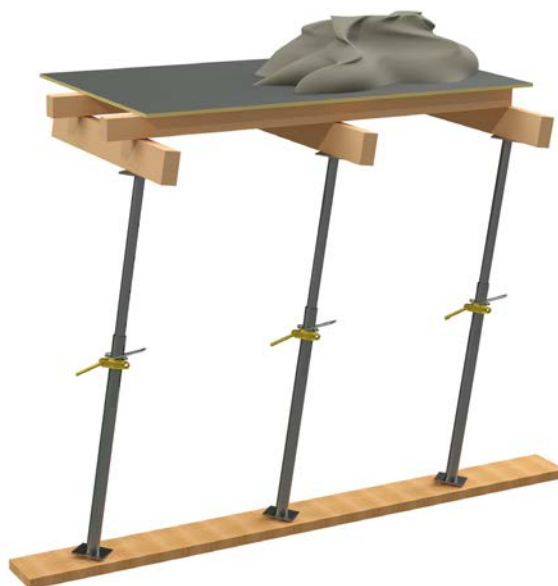
FALSEWORKS MAY INTEND TO TURNOVER AND OR SLIDE IF IT IS SUBJECT TO UNEVEN LOADS
