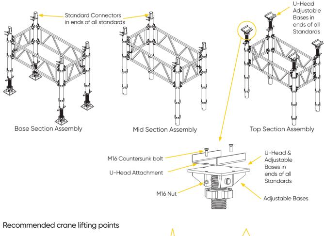
For single Standard 4 legged towers: Wrap under U clusters below top chord of bracing frames with 4 flat/webbing slings. Pick up from inside the tower with min 60 degree angle to horizontal.
