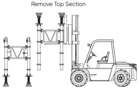
Using mechanical means such as a forklift, lift the top section of the tower clear of the Standard Connectors of the lower section and remove it to a dismantling area. Repeat this process to remove all other sections of the tower.
