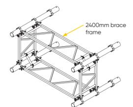
Insert an Adjustable Base into the lower end of each Standard and lock into position using adjustable bolts. Insert a Powershore Standard Connector in the top end of each Standard and lock in position.
