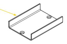
Concrete deposits on U-Head Clean concrete deposits off U-Head paying particular attention to ensure bearing surface is clean and holes are clear.
