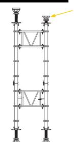
After removal of the soffit formwork check there is at least 400mm of clearance between the top of the Uhead and the underside of the slab. If there is not
