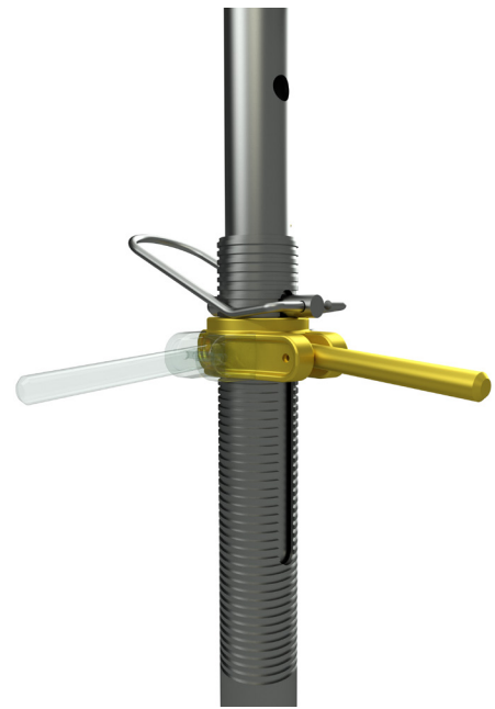
Step 3 Turn the nut handle anti-clockwise for final height adjustment.
