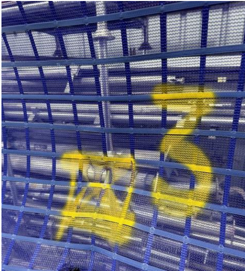
Photograph 5. Detail view of M01- Blue Uni-mesh at point 03 after test.
