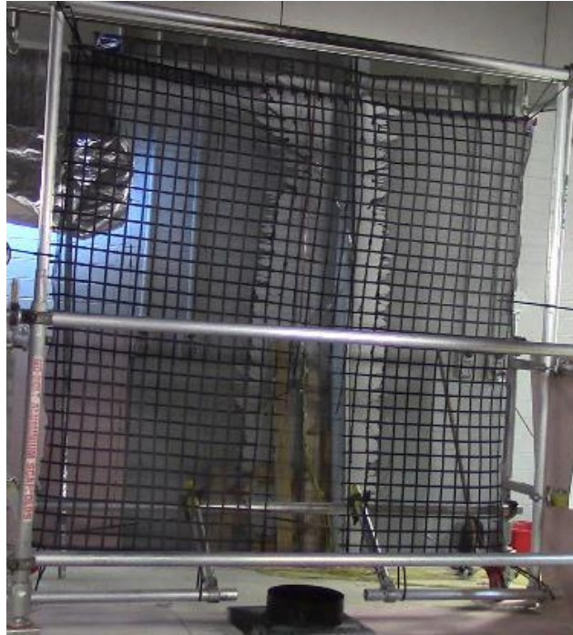
Figure 3 FE3173-1 specimen at t = 6min, 37s. Heptane fuel tray burn out. No flames on the specimen observed.
