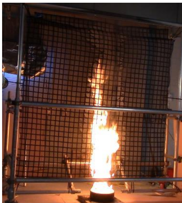
Figure 2 FE3173-1 specimen at t = 1 min 37s showing maximum flame height
