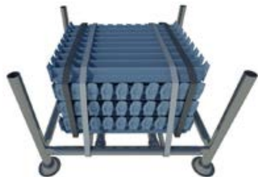
Secure components independently from stillage using at least 2 straps.
