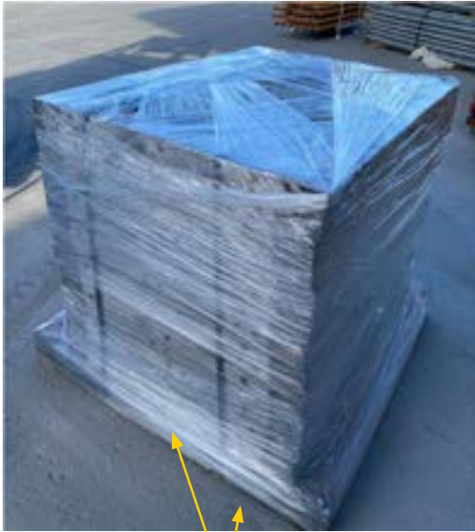
The wrap should cover both the timber pallet and the components.
