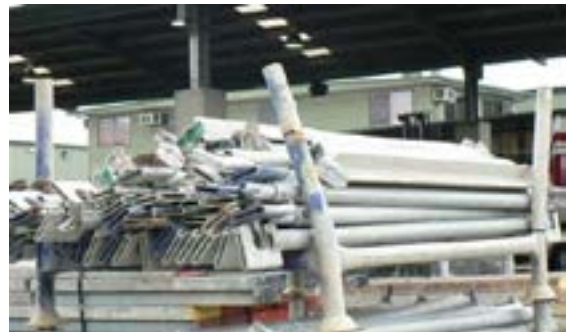
2. Bent vertical leg/post of the stillage.
