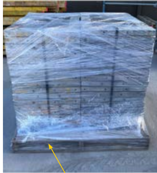
Plastic wrap the pallet and components after completion.
